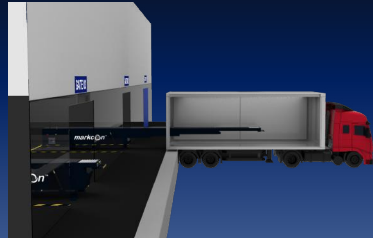
Option-2: where truck touches staging area, hence long extension is required.
