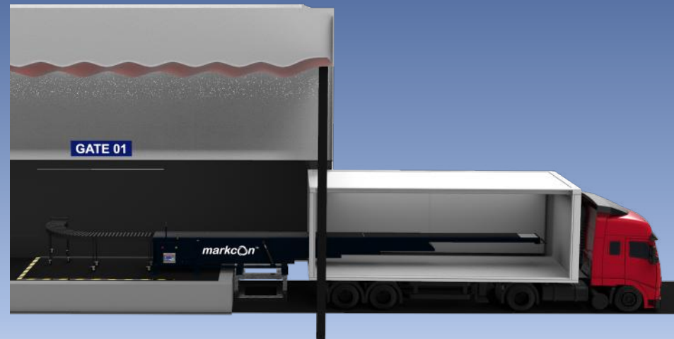
Option-4: Where truck parking is side wise with bay (If no truck bay then stand to be added below the conveyor)
